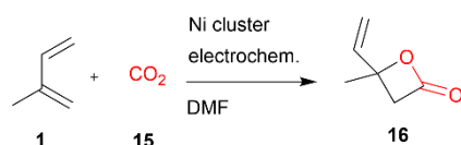
Scheme 4 Electrocatalytic CO 2 capture for the formation of \beta propiolactones
