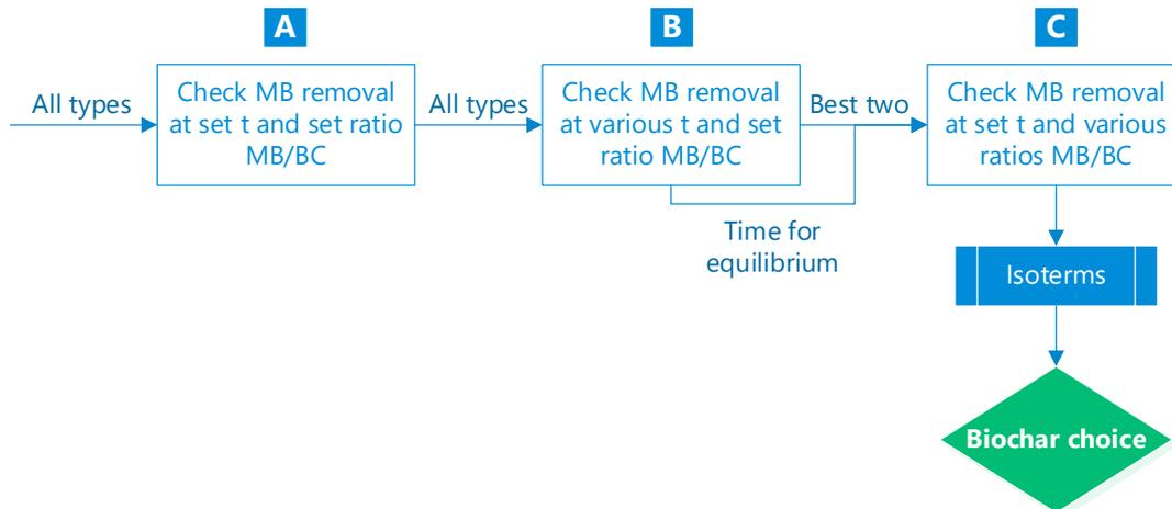
The first trial of tests, here referred as A, had the goal to see how each biochar would act as an adsorbent and how much of the methylene blue they could remove. For this test, 0.1 g of each biochar was added to 20 ml solutions of 12 mg/L of MB with a set contact time (CT) of 2 hours (the detailed methodology can be seen in Appendix A)
