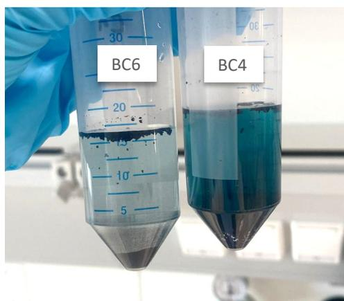
As for maximum capacity at saturation, BC6 outperforms again BC4. However, for the real application, i.e. glyphosate and manganese removal, the concentration will be low as the those micropollutants are found in ranges of  $\mu\text{g/L}$  in the targeted water. Nevertheless, the biochar was tested for MB removal, meaning that the removal performance and its saturation by glyphosate and manganese are unknown.
