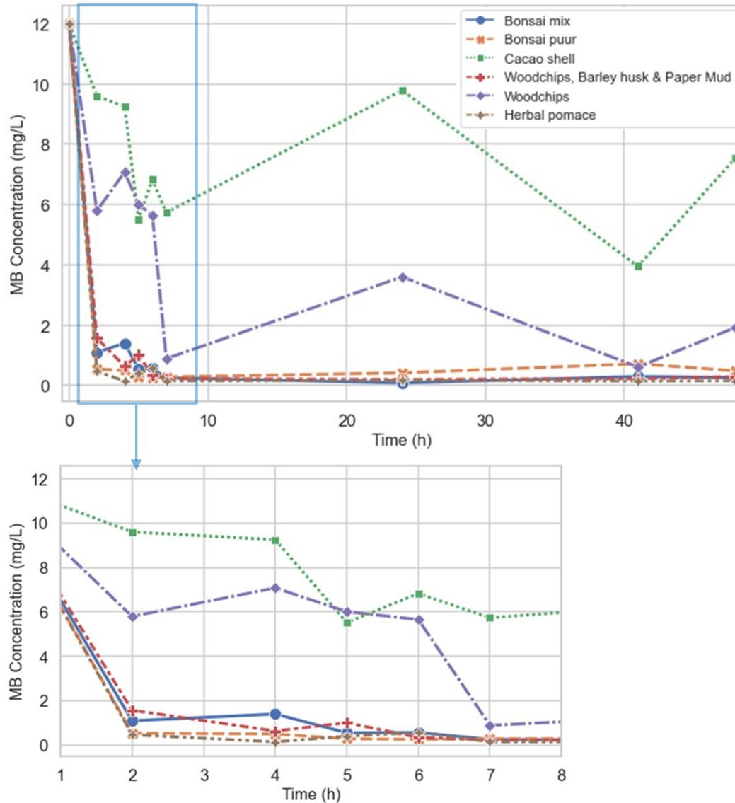
The least performing biochar were BC3 and BC5 (cacao bean shell and woodchips, respectively), which are the coarser and larger types among the tested. This is probably the cause of the lower adsorption, because it provides a smaller surface area, which is known as directly proportional to the adsorption capacity. Besides that, the adsorption is not stable, as concentration peaks are seen at longer contact times, i.e. 24 and 48h, suggesting that desorption occurred.
