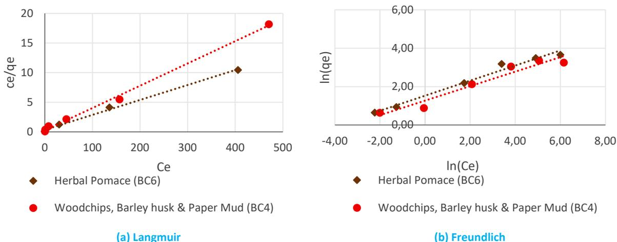
The Langmuir and Freundlich parameters were extracted from the graphs, in Figure 6, by using the methodology contained in Appendix B. The results are showed in Table 3.
