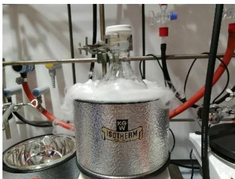
FIGURE 25: REACTION STEP UNDER LIQUID NITROGEN
