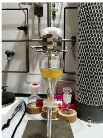
FIGURE 16: EXTRACTION FROM THE DIMETHYLACETAMIDE
