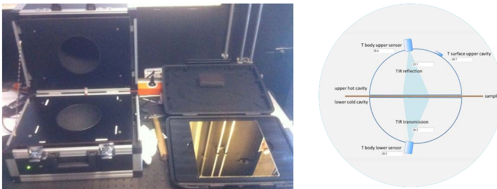
Figure 9 Picture and schematic drawing of the emissivity measurement device (TNO emissivity device).
