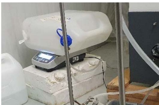
Figure 4 Tank from which water flows to the humidifier on a scale.
