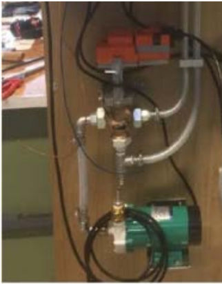
Figure 6 Mixing valve to control the cooling and dehumidification and the scales that measure the water balance.
